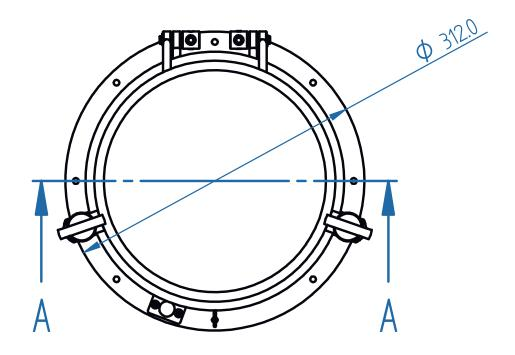
MADE IN STAINLESS STEEL AISI 316 L FINISHING MIRROR POLISHED PLATE DIMENSION ACCORDING CLASS OPTION FIXED TYPE OTHER DIMENSIONS ON DEMAND
