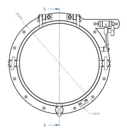
MADE IN STAINLESS STEEL AISI 316 L FINISHING MIRROR POLISHED PLATE DIMENSION ACCORDING CLASS OPTION FIXED TYPE OTHER DIMENSIONS ON DEMAND
